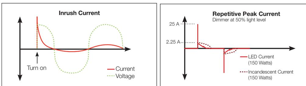
FIGURE 7: Inrush Current and Repetitive Peak Current
